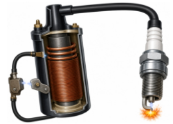
Figure 4-5-7 · A cutaway automotive ignition coil, with a few thick primary turns over many fine secondary turns on an iron core, sends high voltage through a single insulated lead to a spark plug, where a blue-white spark jumps the electrode gap and ignites a flame kernel at the instant the breaker contacts in the primary circuit spring apart.
