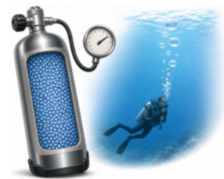
Figure 1-2-5 · A rigid steel scuba cylinder holds a fixed volume of densely packed air molecules at high pressure, while the diver's exhaled bubbles grow larger as they rise toward the surface and the surrounding pressure falls.
