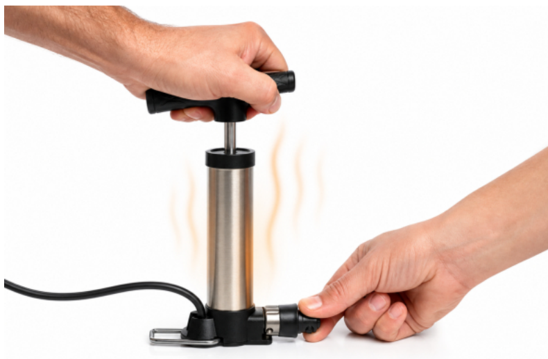
Figure 1-5-1 · A sealed bicycle pump: a fingertip caps the nozzle while the plunger is pushed in, compressing and warming the trapped air.
