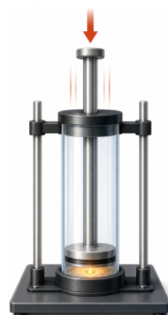
Figure 1-5-5 · A fire piston: driving the piston down fast compresses the trapped air adiabatically, and the temperature soars enough to flash the cotton into flame.
