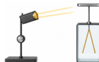
Figure 5-1-2 · Bench setup: a lamp on a stand with a brightness control and a swappable visible/ultraviolet source, aimed at the zinc plate of a gold-leaf electroscope.
