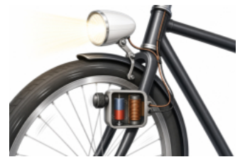
Figure 4-4-8 · A bicycle dynamo: a spinning magnet changes the flux through a coil, inducing an emf that lights the lamp.
