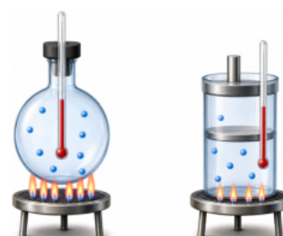
Figure 1-6-2 · The same gas in a rigid flask (constant V ) and in a piston cylinder (constant p ), each with a thermometer and warmed by an identical heater.
