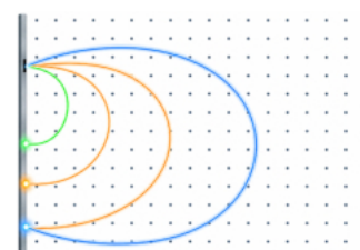
Figure 4-3-7 · A mass spectrometer: ions of the same charge but different mass follow circular arcs of different radii, the heaviest curving least.
