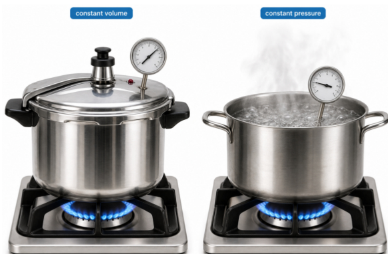
Figure 1-6-1 · The same heat under a sealed pressure cooker (constant volume) and an open pot (constant pressure). In the kitchen the sealed pot runs hotter because trapped steam raises the boiling point; for a gas, because it spends none of the heat on expanding.
