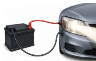
Figure 2-3-6 · A 12-volt car battery drives current around a complete circuit to light the headlamp, which glows and casts a forward beam while the wires and battery themselves stay dark.
