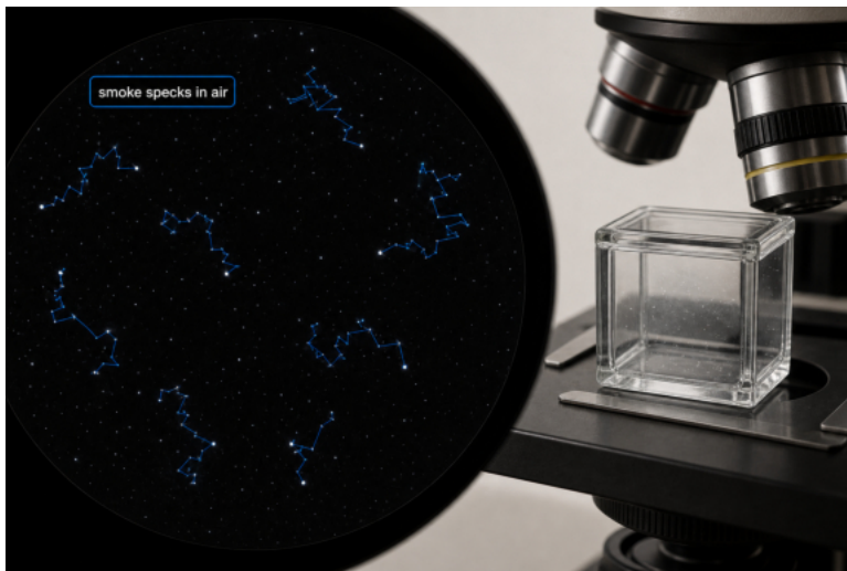
Figure 1-3-1 · Smoke specks under a microscope never rest: air molecules strike them unevenly from every side, and those same countless impacts, spread over a wall, make up pressure.
