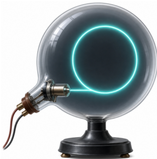
Figure 4-3-1 · With the field off the electron beam runs straight to the screen; switch on a field into the page and it curls into a circular path.
