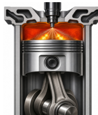
Figure 1-5-4 · At the top of a diesel engine's compression stroke, air squeezed into a small, glowing-hot space ignites the fine cone of fuel sprayed from the injector, with no spark plug needed.
