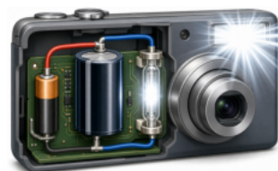
Figure 2-6-6 · A small battery slowly charges a large capacitor, which then dumps its stored energy in a single sudden burst through the flash tube to fire the camera's flash.
