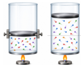
Figure 1-6-4 · Two identical gas samples are heated equally: the locked left piston keeps the volume constant, while the free right piston rises above its original level as the gas expands at constant pressure.
