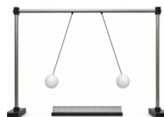
Figure 2-1-2 · Two like-charged foam balls on insulating threads hang from a rod and settle apart; a ruler reads their separation r .
