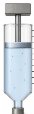
Figure 1-1-2 · A sealed syringe held vertically: a known load presses the plunger while the trapped volume V is read on the barrel scale; the nozzle is capped.
