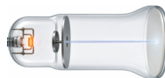
Figure 2-5-5 · Inside an evacuated tube, particles leave the hot filament almost at rest and are accelerated through the hole in the anode plate into a fast, straight beam that travels to the screen.
