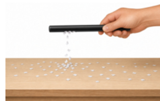
Figure 2-1-7 · A charged rod lifts only the paper scraps directly beneath it while scraps a short distance away stay flat and undisturbed, showing how steeply the electrostatic attraction weakens with distance.
