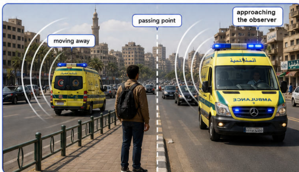
Figure 2-8-1 · The pitch is higher as the ambulance approaches and lower as it recedes.
