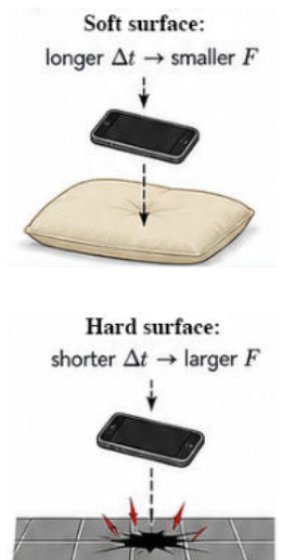
Figure 1-7-7 · A hard surface shortens the contact time and raises the force.
